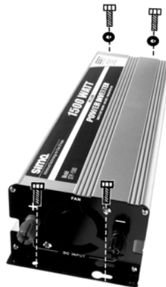
Figure 2, Mounting the power inverter
