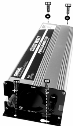
Figure 2, Mounting the power inverter
