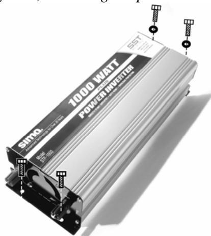
Figure 2, Mounting the power inverter
